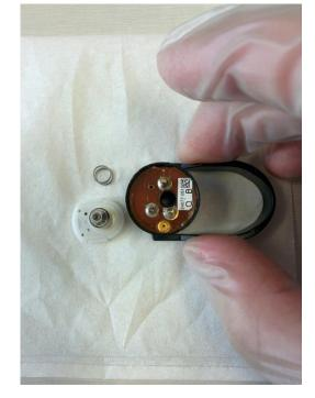
**Note:** Discarding the PID electrode stack:
